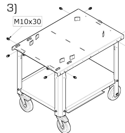
Screw stand legs to the top plate. Do not tighten the joints.
