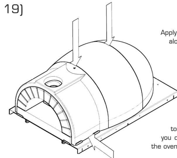
Apply silicone caulk between the body parts and along oven circumference between the bottom edge of the body and the stand - into the formed joint, the used dilatation pads should also get fixed. Silicone the chinks in the way the silicone caulk could be removed in the case of necessity of disassembling the oven (e.g. in the case of a warranty claim).
