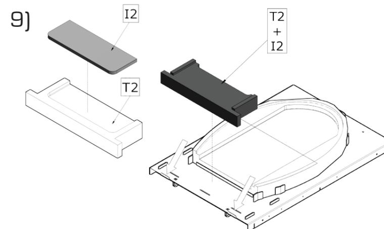
Cut the gum pad P12 (1 mm thick) according to the size of the front stopper and glue it to the inner side of the stoppers using the silicone caulk.
