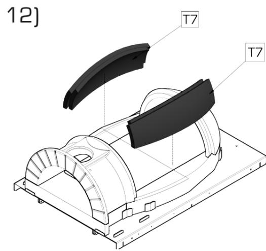
Place the small side arch between the front and rear arch. Side arches should be placed with a hole towards the front portal.
