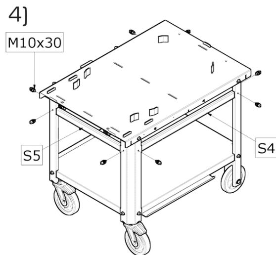
Bolt partitions between individual legs (direct the bends inwards). Tighten all the already applied bolted joints.
