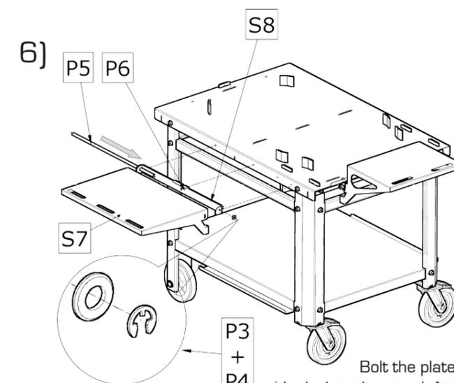
Bolt the plate for the side desk to the stand. Attach the desk to the plate by pulling the axis through and securing it on both sides against slipping out by washers and lock rings. The side to which the side shelf is to be mounted may be selected as necessary.
