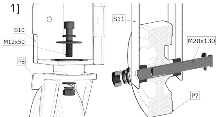
Bolt the wheels to the stand legs according to the illustration. Insert spacers between the fixed wheel [P7] and the wheel axis (short spacers). Put the wheel axis together with a guide tube (long one) through these spacers. Place washer, spring washer and nut on the axis and tighten it.
