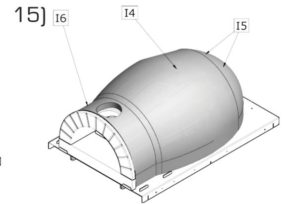
Cover the assembled arch with at least 1 layer of aluminium foil. Place the isolation bio-mat on the aluminium foil according to the cutting plan for the bio-mat. Make sure the bio-mat doesn't get distorted during the application.
