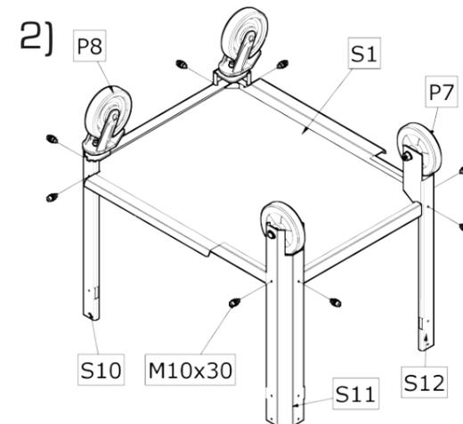
Bolt the bottom plate to the stand legs. Do not tighten the joints. In case the a screw doesn't easily fit into a hole, make the hole wider with a file. Paint over the altered surface with a paint for metal.
