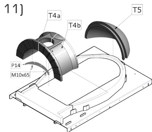
Place the front arch on the front plate of the bottom. Then bolt the smoke guard to the arch. Do not tighten the joints too firmly, otherwise the damage of the refractory shapes may occur due to heat dilatation. Place the rear arch on the rear plate of the bottom.
