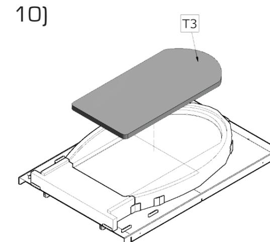
Place the inner plate into the bottom plate cutout.
