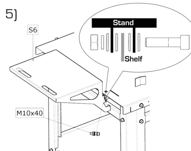
Insert the front shelf into the grooves and bolt it on both sides. Do not tighten the joints too much, movement of the shelf in the grooves needs to be secured so that it can tilt.
