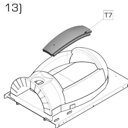
Place the central part of the arch with a hole towards the chimney. Shape should be placed on the top of the arch.
